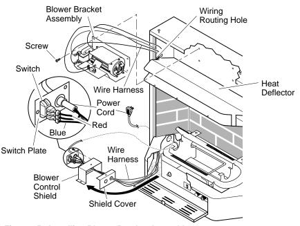
Figure 15 - Installing Blower Bracket Assembly
